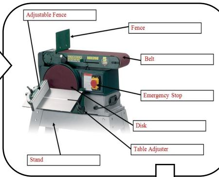
**Table-** This can be adjusted on most belt and disk sanders between the angle of 0 and 45 degrees using the **table adjuster** knob. In the diagram (above) this belt and disk sander has an **adjustable fence** which can slide up and down the table. The angle can also be changed.
