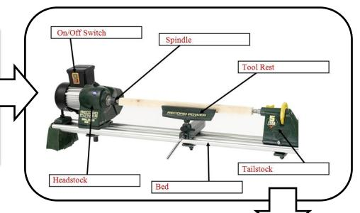
**Bed-** This is a horizontal beam which holds together the basic components.
